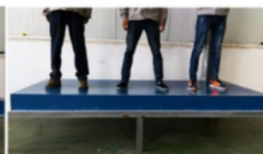
No deformation with 210KG
