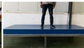
No deformation with 62KG
