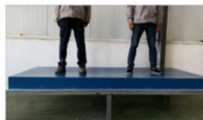
No deformation with 140KG
