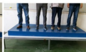
No deformation with 300KG
