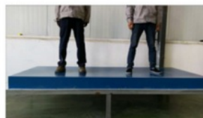
No deformation with 140KG
