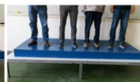
No deformation with 300KG
