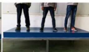
No deformation with 210KG
