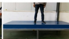
No deformation with 62KG
